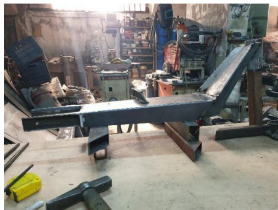
Figure 6.5 Welding the Handlebar stem seat to the 'Neck'
