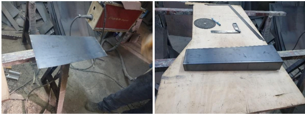
Figure 6.1 Cutting the sheet in the dimensions determined and bending
