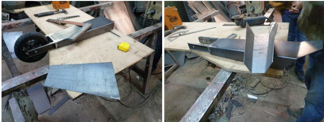
Figure 6.3 Bending the neck of the main part
