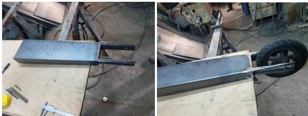
Figure 6.2 Welding the fork and optimizing the wheel arch
