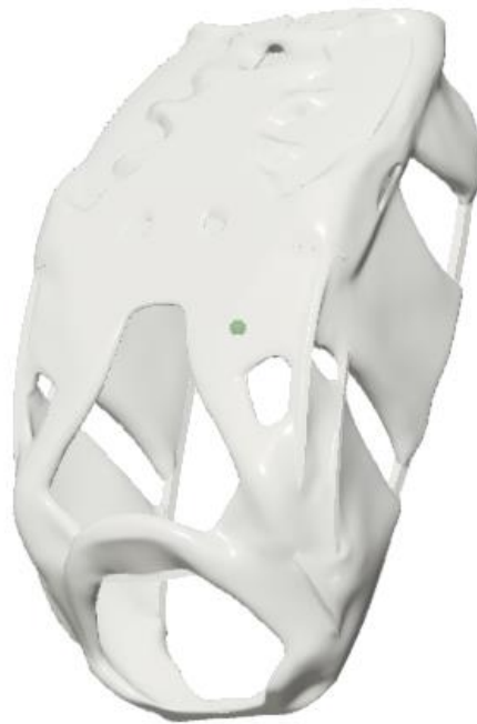
Figure 13 Generative Designed Gaming Mouse Perspective View
